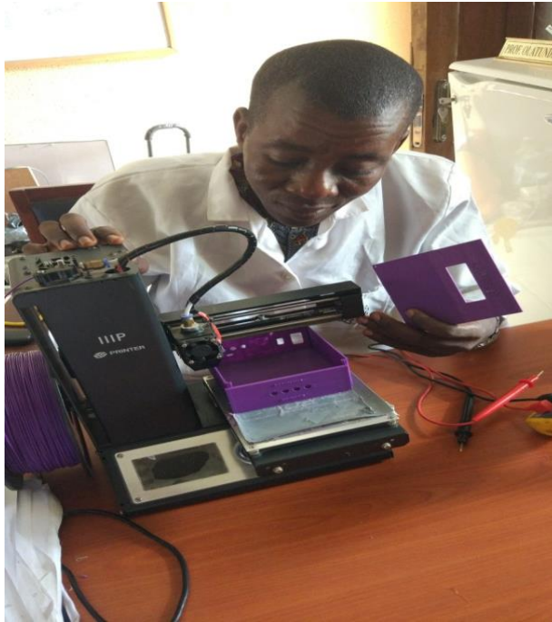
Figure 3: The printing stage of the plastic case with 3D testing printer
